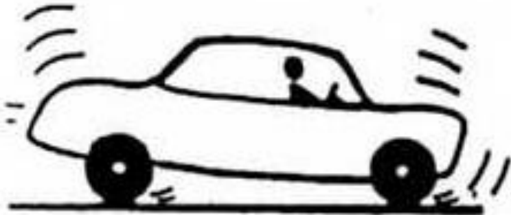
FIGURE II-120 Action of car as brakes are being applied in the road test. (Courtesy of Monroe Auto Equipment Co.)
